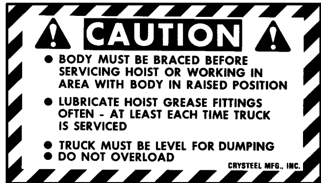
400643—Mount on the longbeam on the drivers side.
