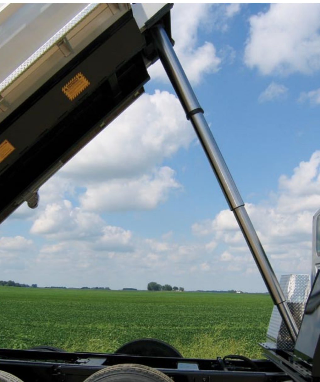
Crysteel Marathon's ingenious body mount lifts directly on the longbeams for efficient power delivery and superior stability, throughout the dump cycle.
