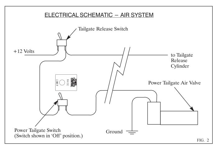
Connect a 16 gauge wire from the switched side of the Tailgate Release Switch to the common terminal of the Power Tailgate Switch. Connect a 16 gauge wire from the switched side of the Power Tailgate Switch to one of the wires on the Power Tailgate air valve. Connect the other wire on the air valve to ground.
