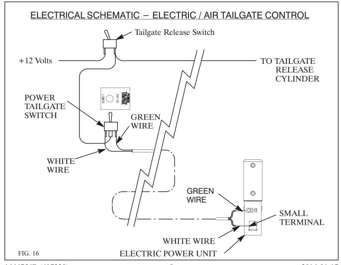
Connect a 16 gauge wire from the switched side of the Tailgate Release Switch to the common, middle terminal of the Power Tailgate Switch. The electric power unit has a two wire, 20 foot long cable prewired to the power unit. Route the free end of the cable into the cab of the truck. Connect the white and green wires to the Power Tailgate switch - white wire to raise the tailgate, green wire to lower the tailgate.
