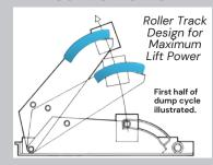
At beginning of cycle, short arm position of roller allows almost 1/3 more breakaway power to start heavy loads. As load rises, roller moves along its track, increasing effective length of upper hoist arm. When roller reaches end of track, hoist automatically becomes scissors-type hoist, with enough power to easily finish dump cycle.
